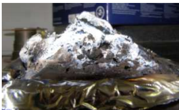
Figure 7. Residue of TPU/ZnO composite after a cone calorimeter experiment. Note it exhibits an intumescent behavior.
