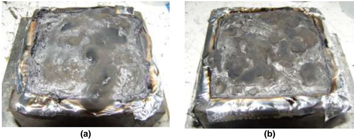
Figure 10. Residues of TPU/APP (a) and TPU/APP-MWNT nanocomposite (b) after a cone calorimeter experiment (external heat flux = 35 kW/m 2 ).
